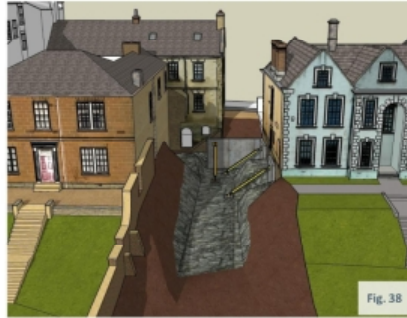
2) Basement walls cast against existing buildings in sections, leaving existing rock between sections to provide support
